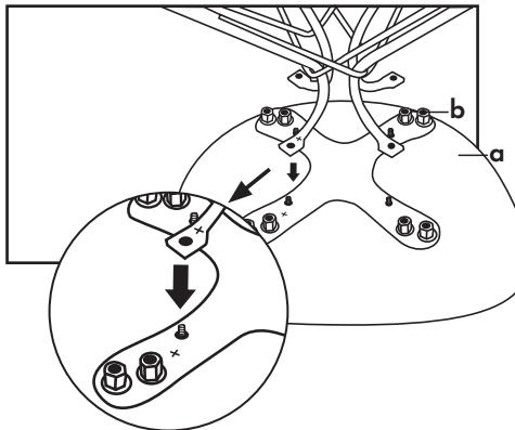
**2** Attach the nuts (b) to the screws available under the seat.
