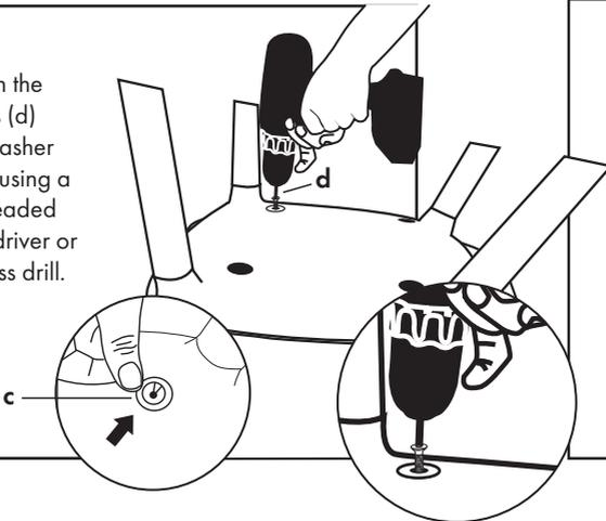
**!** Please be sure not to miss any screw holes and fasten all screws equally and tightly. Otherwise, you may face breakage or cracking during the time of usage.
